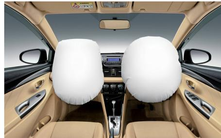
The National Highway Traffic Administration: Tens of millions of vehicles with Takata air bags are under recall. Long-term exposure to high heat and humidity can cause these air bags to explode when deployed. Such explosions have caused injuries and deaths. NHTSA urges vehicle owners to take a few simple steps to protect themselves and others from this very serious threat to safety.
